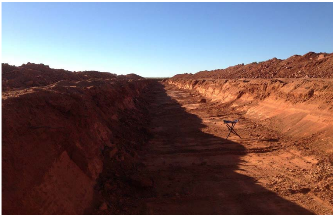
Figure 3. Gold-bearing vein material and waste extracted from 240 metres of strike length (first bench) at the Western Limb. Material on the left surface is stock-piled high-grade vein, and on the right is waste material or material being resampled to check for presence of gold.
