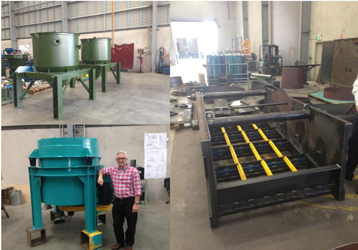
Photograph 4. Top Left - Concentrate hoppers, Bottom Left - Knelson Concentrator (Chairman - Mike Etheridge pictured) and Right - Screen Deck all being built at Consep in Sydney.
