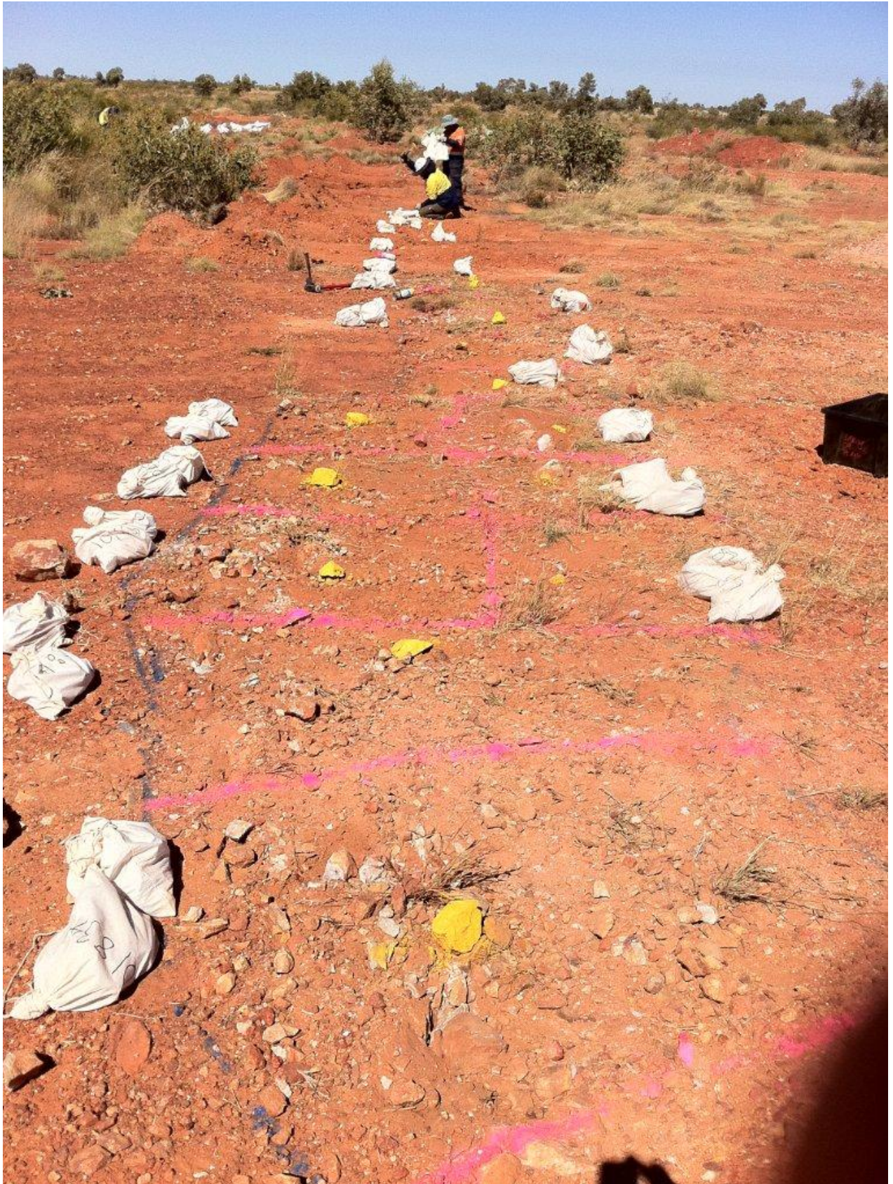
Figure 3 - Gridded and sampled vein (pink lines represent grid boundaries of vein samples).
