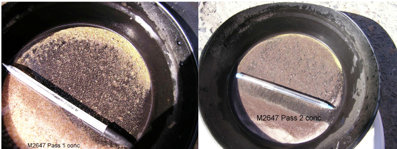
Figure 5 - Gold Pan concentrates from Knelson Concentrator test work. Left = First Pass concentrate from 220 micron grind. Right = second pass concentrate from 113 micron grind.
