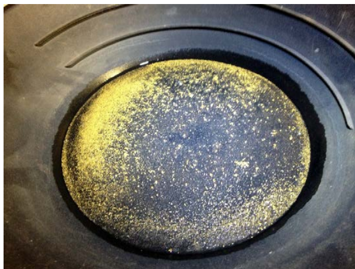
Figure 7 - A total of 12 grams of gold panned from 15kg of material indicating a grade of at least 800g/t gold with the laboratory assays likely under-calling the overall grade.
