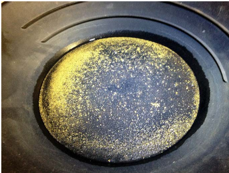
Figure 1. A total of 12 grams of gold panned from 15kg of material from hole GHRC100014 indicating a grade of at least 800g/t gold with the laboratory assays likely under-calling the overall grade.
