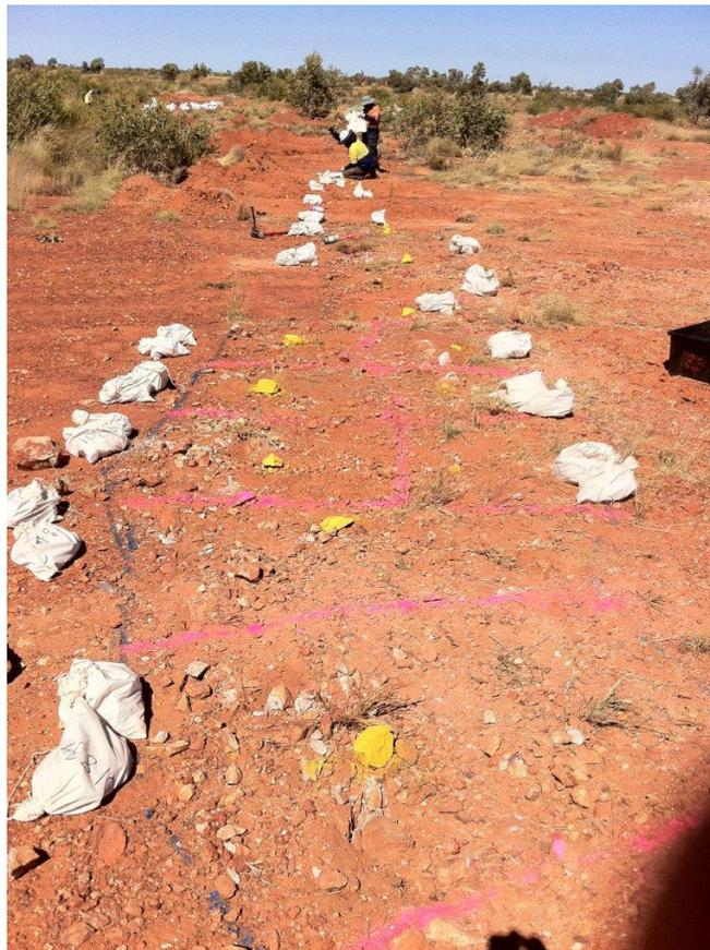
**Figure 6. Gridded and sampled vein (pink lines represent grid boundaries of vein samples) at Old Pirate**
