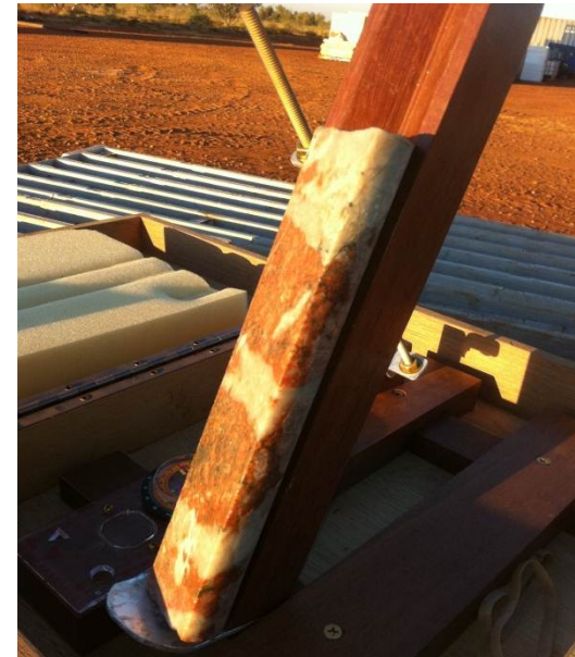
Flat lying grey quartz veins with visible gold. Up to 60g/t Au over narrow widths.
