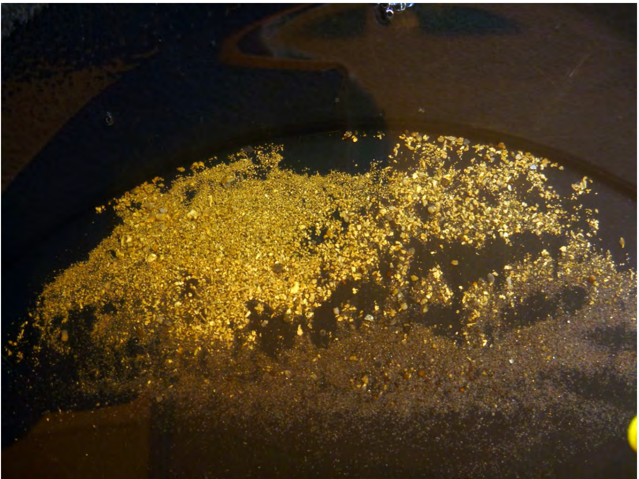
Figure 7. High grade gold panned from split RC drill sample from hole OPRC100021
