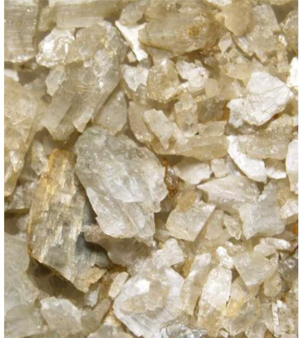
8.10%  $\text{Li}_2\text{O}$  Spodumene from HLS Testwork
