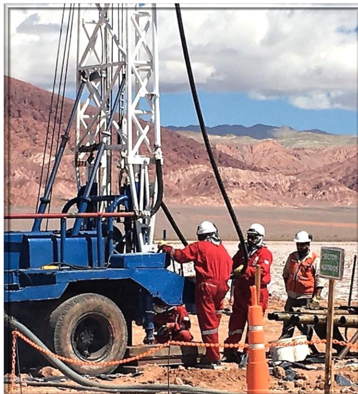
Images of the rotary drill rig adjacent to the second drill hole of the Kachi project
