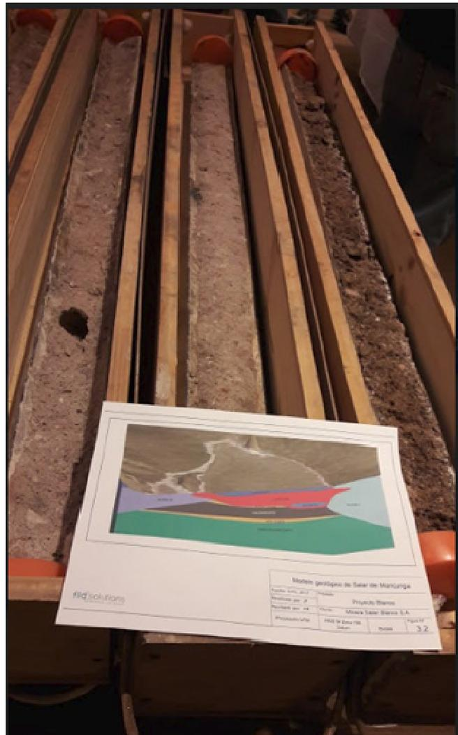
reason for this was to maintain as much of the liquid in the core to gauge the porosity of the material and to minimize the contamination that arises from the use of drilling mud and fluids in other drilling techniques.
