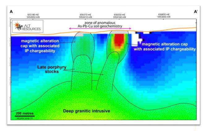
Figure 6. Cross-section of a conceptual model for the Windy Hill area. This demonstrates the relationship between a deeper intrusive body, later porphyry intrusive stocks rising to shallow levels, as well as the observed magnetic and IP responses. The base image is a vertical slice through the magnetic model, along line A-A' shown on Figure 4.
