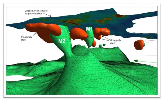
Figure 9. 3D image of the magnetic model (green shell at 143 Si units), IP model (red shell at 37 mv/V) and gridded arsenic anomalism in soils at surface. The view is to the south-west, looking obliquely upwards towards the ground surface. This image clearly demonstrates the close relationship between the M1 and M2 magnetic anomalies, and IP anomalism, as well as anomalous arsenic in soils at surface.
