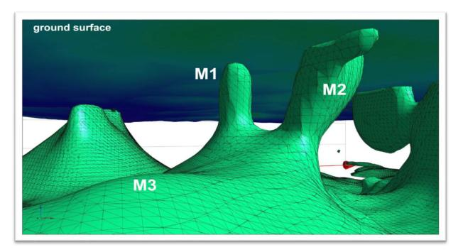
Figure 2. 3D view of the Windy Hill magnetic model. Surfaces are at 135 SI units. Key magnetic anomalies are labelled M1, M2 and M3. The view is to the North-North-East, looking up at the surface from below ground. No scale is given due to the variable distances produced from a 3D image projected onto a flat surface. The anomalies M1 and M2 are approximately 300m apart. Refer to Figure 3 for a scaled map in plan view.
