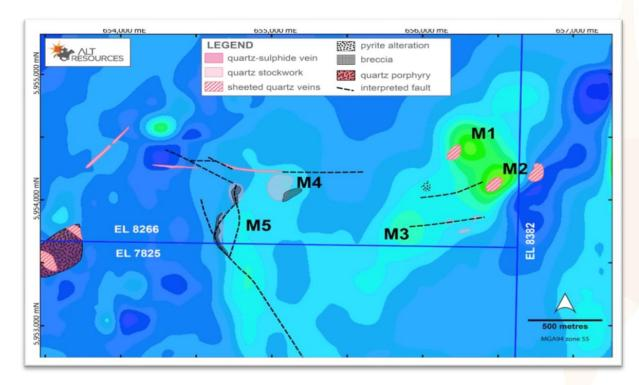
Figure 3. Horizontal slice through the magnetic model at Windy Hill, at 600m RL (between 200-300m below surface), overlain by mapped geology. The key magnetic anomalies are labelled M1-M5. The relationship between magnetic anomalism and known mineralisation features at surface is evident.
