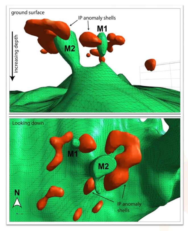
Figure 5. 3D image of the magnetic model (green shell at 143 Si units) and IP model (red shells at 37 mv/V). The view in the top image is to the south-west, looking obliquely upwards towards the ground surface. The bottom image is looking directly down. These images clearly demonstrate the close relationship between the M1 and M2 magnetic anomalies and enveloping IP anomalism.
