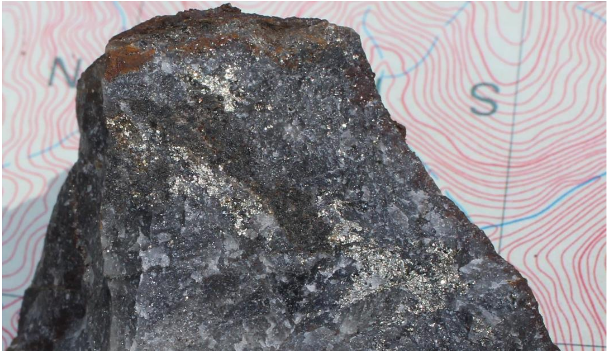
Figure 2.5 Mineralised chert-ironstone sample from the Pine Creek lode
