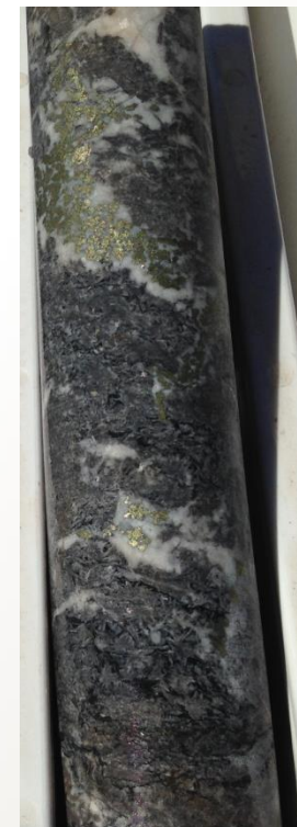
Drill core CCD02, evaporite horizon, disseminated chalcopyrite. Visible ex-gypsum crystals of evaporite horizon
