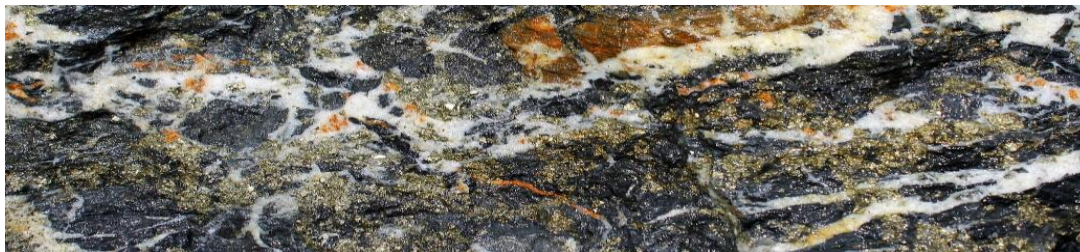
Brecciated shales with quartz fill, disseminated pyrite and bonanza gold grades
