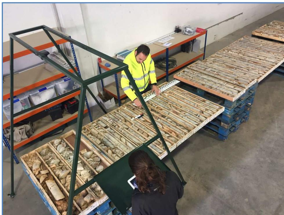
**Figure 3: Diamond drill core being process by Plymouth geological staff at San Jose**
