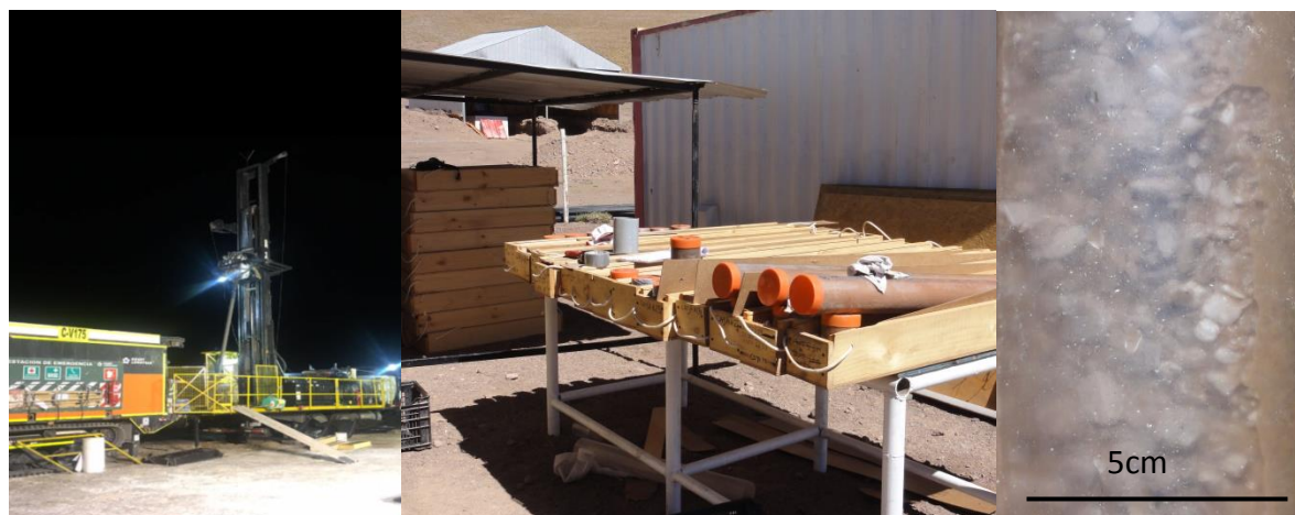
Figure 2: Maricunga Sonic drill rig working at night, cutting porosity core samples and gravel material in core
