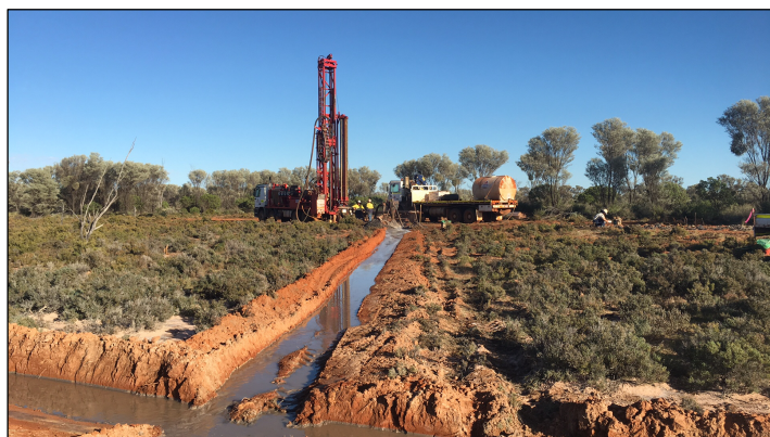
Figures 5 & 6: Right, piercing the basal sand layer and channeling the natural overflow to containment bund
