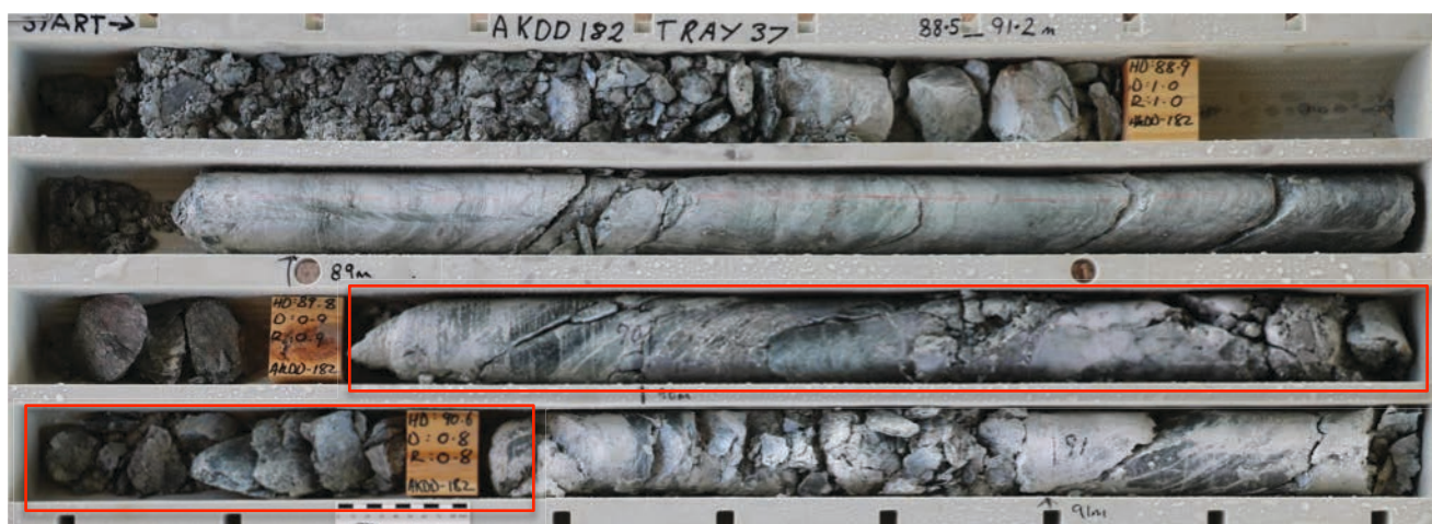
Figure 2 – AKDD182 drill core including intersection of 0.6m @ 0.8% Cu, 44 g/t Ag and 0.8 g/t Au from 89.9m
