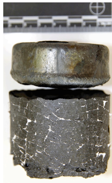
Plate 1: Pig Iron (top) & titanium slag (bottom) produced from Baobab iron ore & local Mozambique coal
