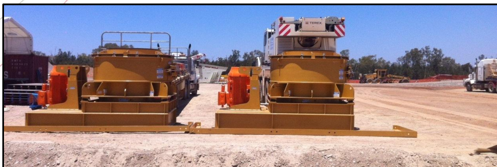
Tertiary crusher bases delivered on site
