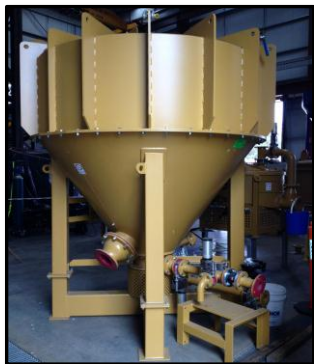
Inline Pressure Jig Completed
