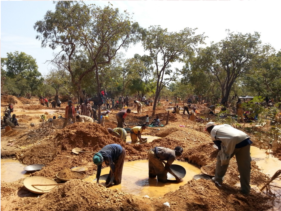
Figure 3: Nangalasso Project – active artisanal mining, recovering gold from shallow clay and panning.
