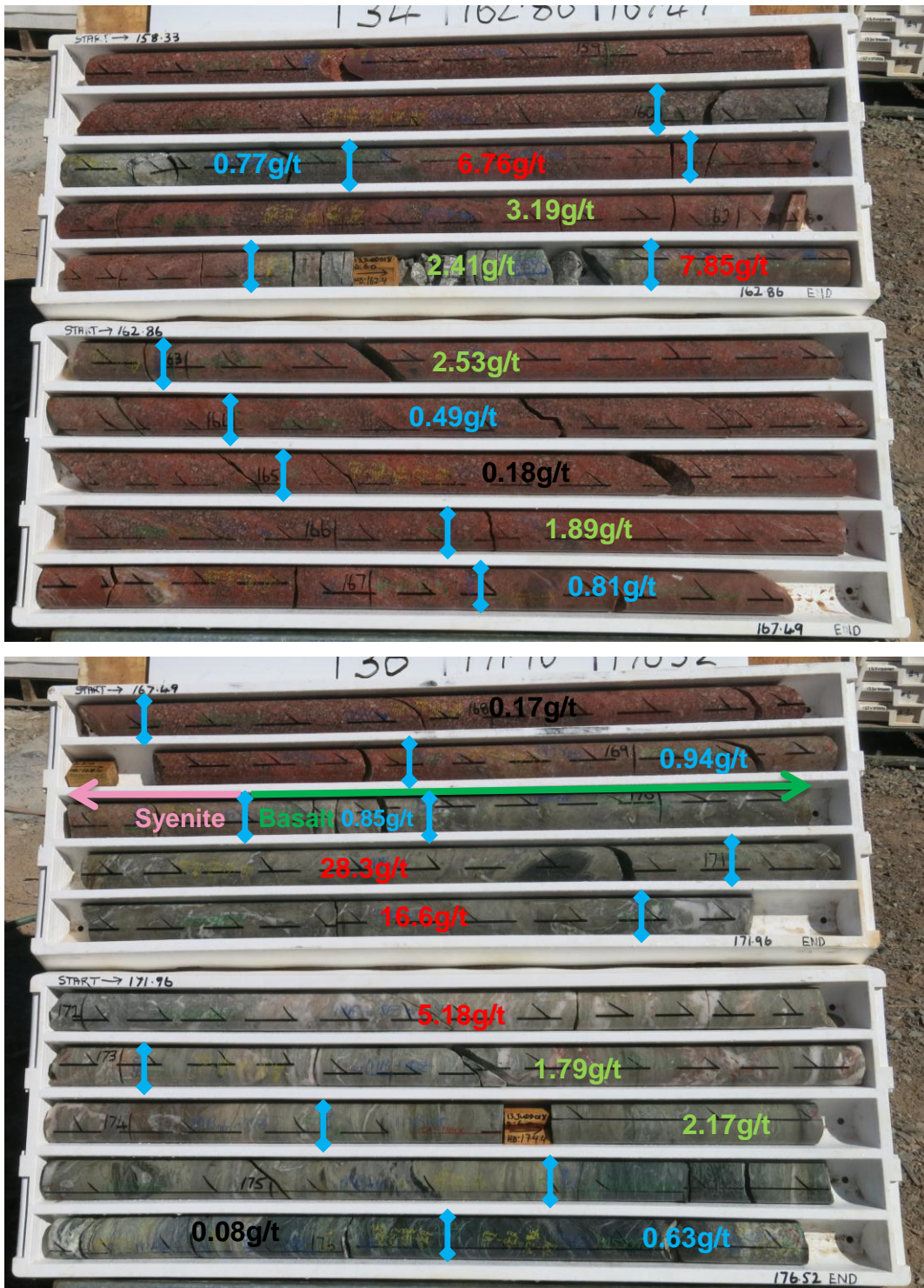
Figure 1: Core photographs and assay values for intersection of 17.2m @ 4.8g/t in 13JURD018 showing high grade gold defined adjacent to the contact of the syenite (See Figure 3 for cross section reference)
