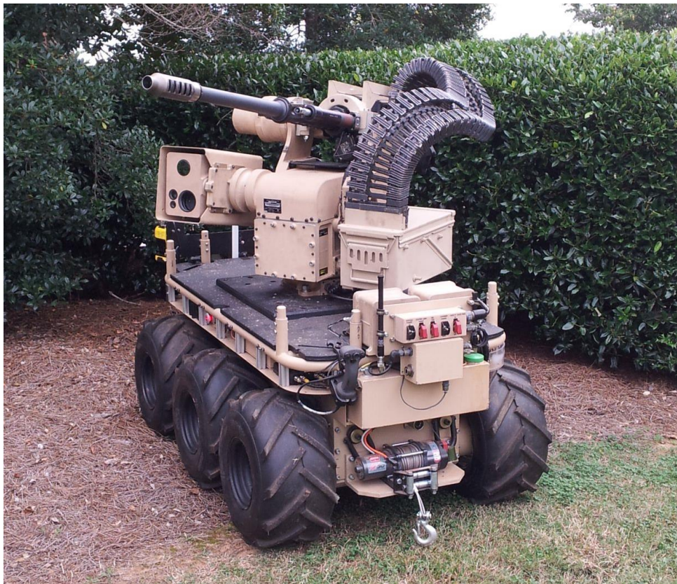
Figure 2: R-400S mounting the ATK M230LF 30 mm cannon. The weapon system is itself mounted on a Northrop Grumman CaMEL military robot.
