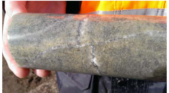
GHD001, 825m – Multi-stage quartz-sulphide veins in sericite-sulphide altered monzodiorite (HQ core diameter – 63.5mm)
