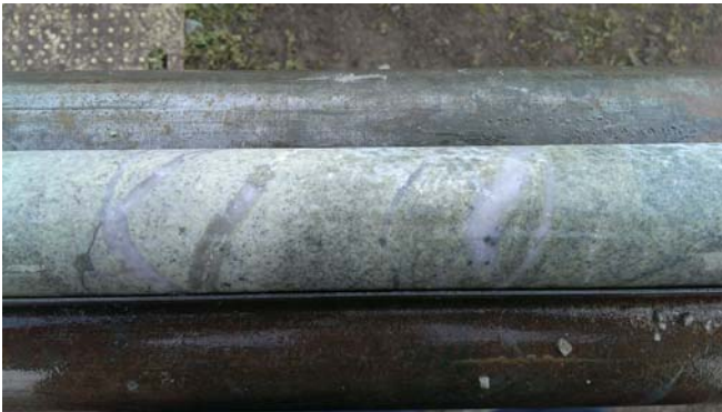
GHD001 around 820m, sulphide-sericite altered monzodiorite exhibiting sheeted veins (HQ core diameter – 63.5mm)
