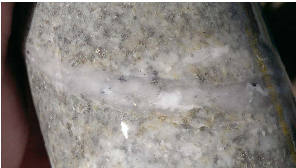
Narrow quartz vein carrying visible gold (bright yellow fleck) and silver coloured sulphides (arsenopyrite and molybdenite) from ~168m (HQ core diameter – 63.5mm)
