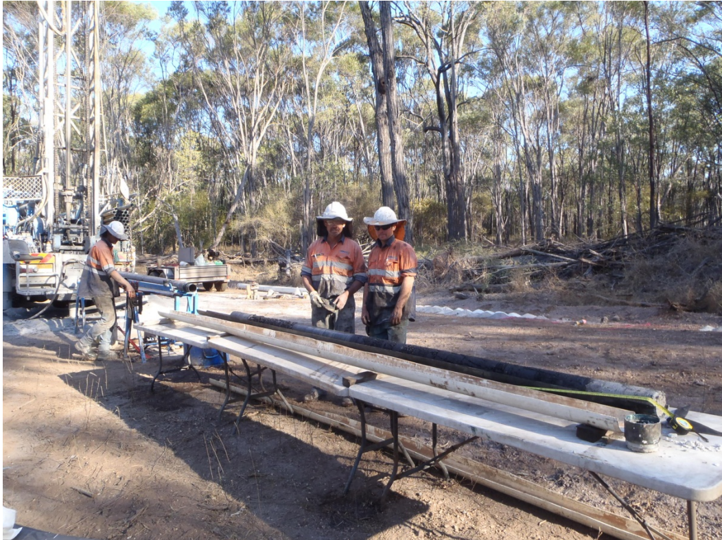
Figure 2: Coring by twinning open PCD hole ML0014, the B4 seam is shown in the photograph
