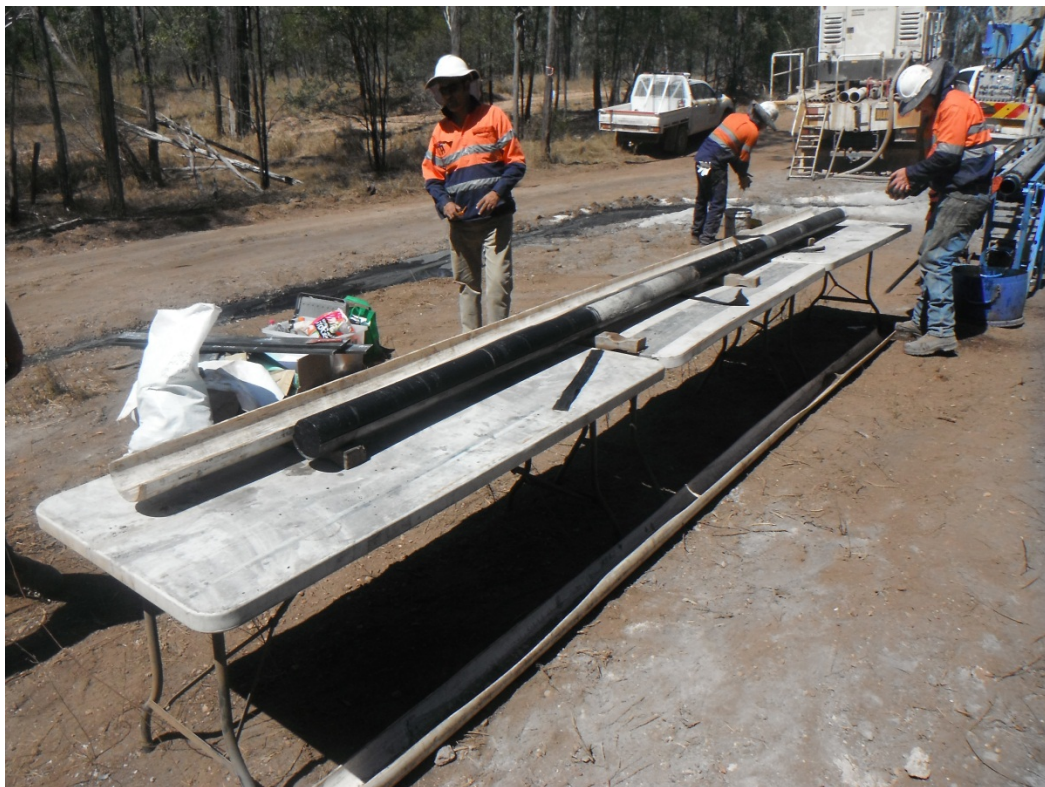
Figure 2: Coring by twinning open PCD hole ML0014, the B7 and part of the B8 seam is shown in the photograph
