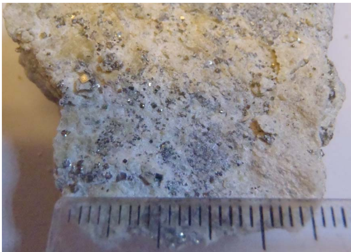
SGRDD014, Piece of core from 24.9 metres ( 15.40 grams/tonne gold from 24-25 metres downhole 1 ). Exposed vein exhibiting disseminated sulphides (stibnite, cubic pyrite and arsenopyrite) in sericite-quartz altered felsic dyke, (scale millimetre divisions).
