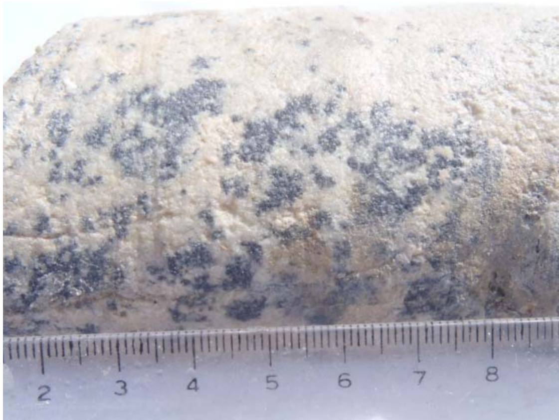
SGRDD014, Core from 24.7-24.8 metres ( 15.40 grams/tonne gold from 24-25 metres downhole 1 ). Blebs of disseminated grey sulphide (stibnite, antimony sulphide) in phyllic altered felsic dyke (centimetre scale). 24-25m downhole 1 contained 0.694% Antimony per tonne, indicating potential for antimony credits.
