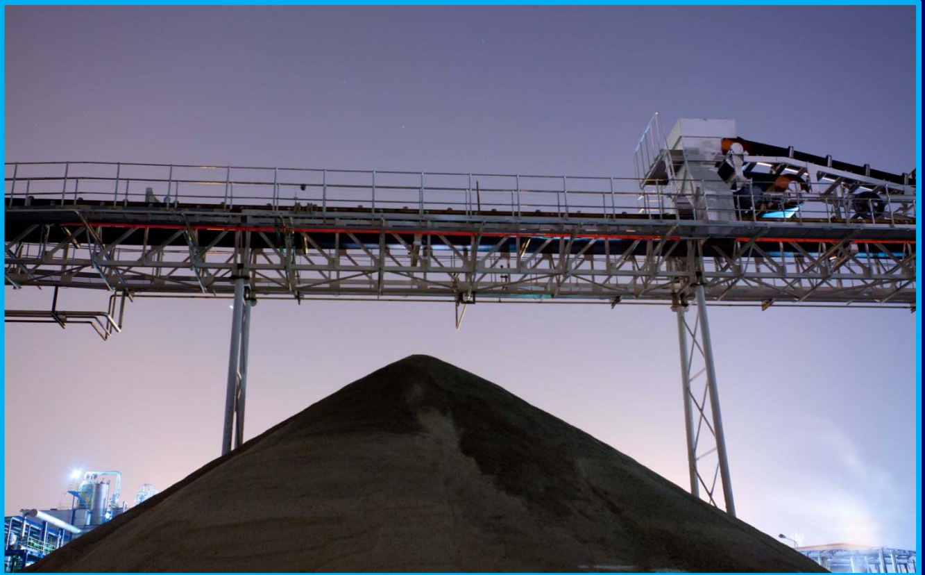
Spodumene unloaded at wharf and conveyed via over land conveyor to the ore storage area
