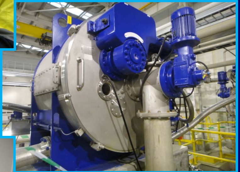
Lithium carbonate centrifuge in operation
