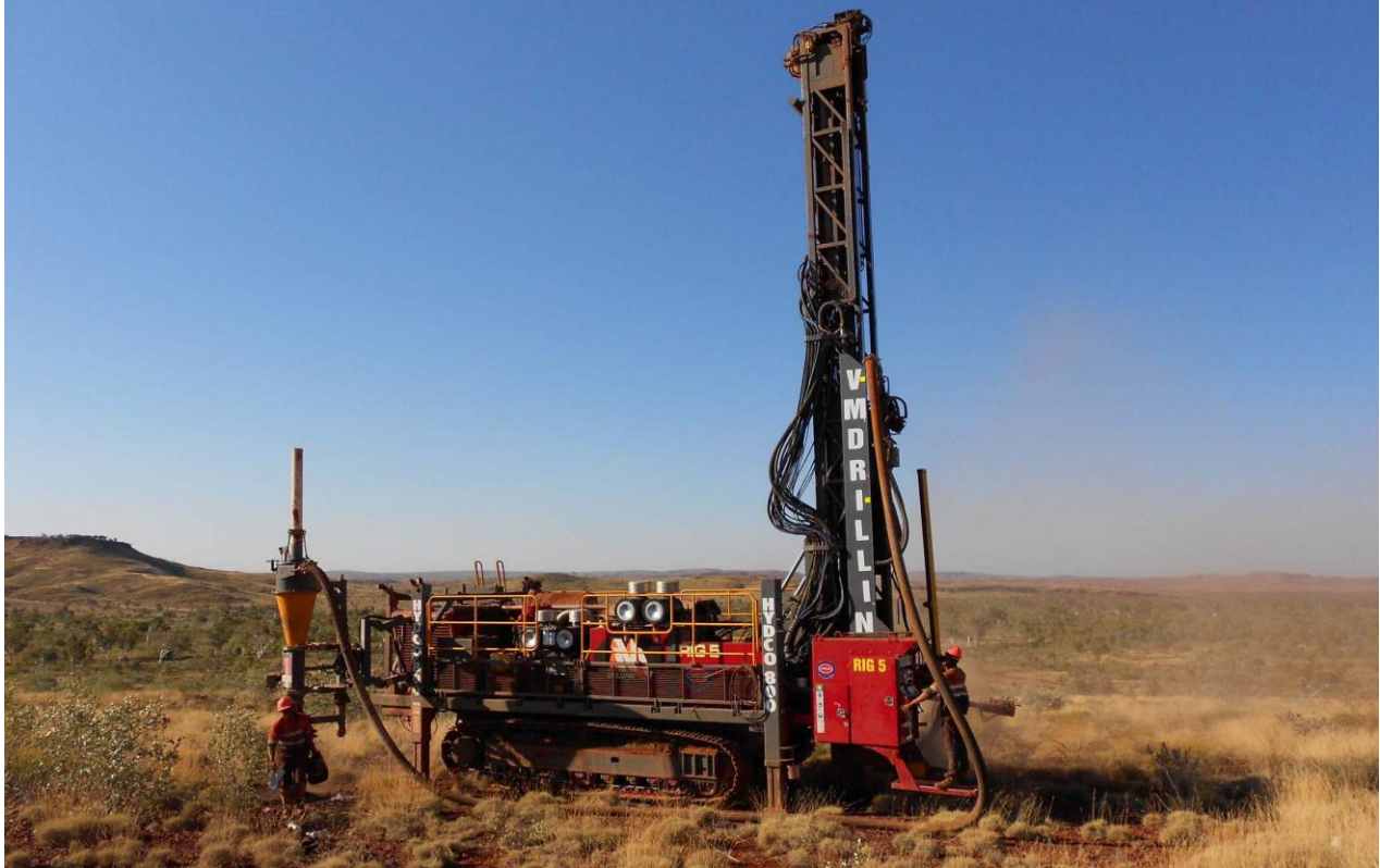
Figure 3: Hydcos 800 Reverse Circulation Drilling Rig operating at the Yandicoogina South tenement.
