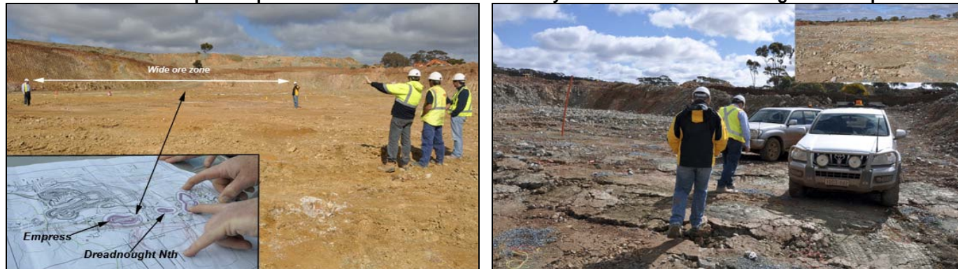
Figure 11. Wide Ore Zone of Empress open-cut , and Neatly Blasted Floor of Dreadnought North Open-cut
