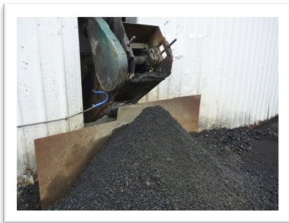
The ash tailings from briquettes have a distinctive black colour. This visual cue in addition to test data from BAIC's lab indicates not all carbon is being combusted in the briquettes
