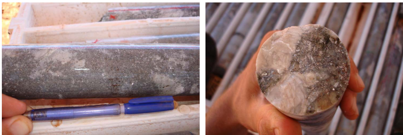
Two photographs of diamond core from Hole ARMCRCD001 showing sulphide mineralisation hosting gold, silver and copper. This hole was drilled 200m west of the main mineralisation at Mt Clement and represents a significant step-out discovery of a new zone of mineralisation.
