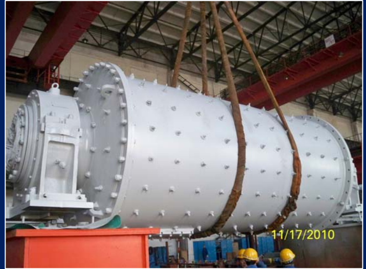
Ball mill fabrication at suppliers workshop
