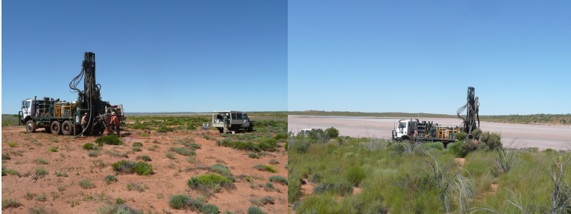
Figure 2. Air Core Drilling on salt lake margins
