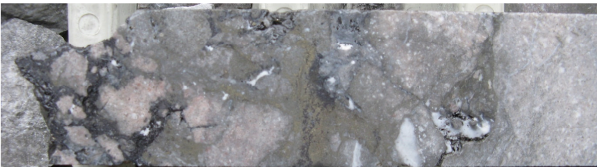
Figure 1. Pyrite-enargite veining in strongly silicified rhyodacite porphyry at 149m in hole HC10RCD941 assaying 30.1 g/t Au, 63 g/t Ag and 2.53% Cu.
