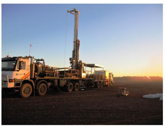
Figure 1, Sonic Drill Rig (Boart Longyear) on Dynasty's Prairie Downs Iron Ore Project
