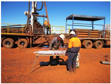
Figure 4, laying out and measuring a sonic drill sample
