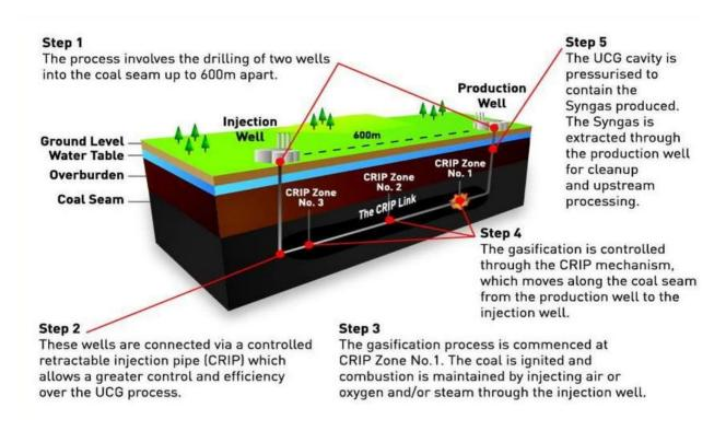
Clean Global Energy's advanced Linear CRIP (Controlled Retractable Injection Point) UCG process provides greater efficiencies and control with less overall operating and capital costs.
