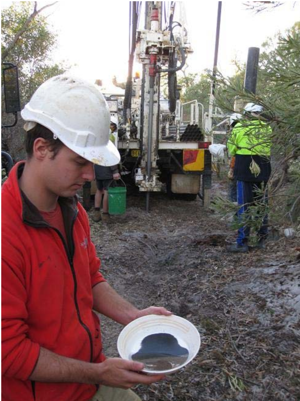
Figure 2 Project Geologist Wayne Carter Panning High Grade HM in Hole GG311
