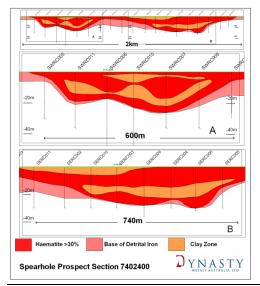
**Figure 5** – Top Section: Full Cross Section 7402400N looking northwards showing the continuity, depth and the lateral extent of the Spearhole Detrital Channel Iron Deposit and areas containing >30% visual Haematite. Thick zones are enlarged in sections A & B.
