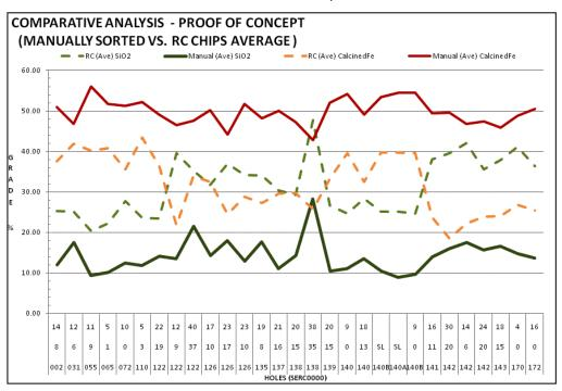
Full results from the proof of concept sampling are attached showing the highly encouraging Fe grades. These include up to 60.96% Fe from the magnetite fraction from a surface sample taken from near the collar SERC055.
