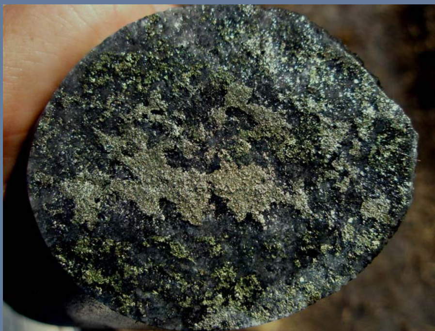
Figure 6: Pyrite and Chalcopyrite in magnetite vein at 149 m depth in Peenam Hole PEED1 The magnetite association implies that the best mineralisation will lie within magnetic anomalies
