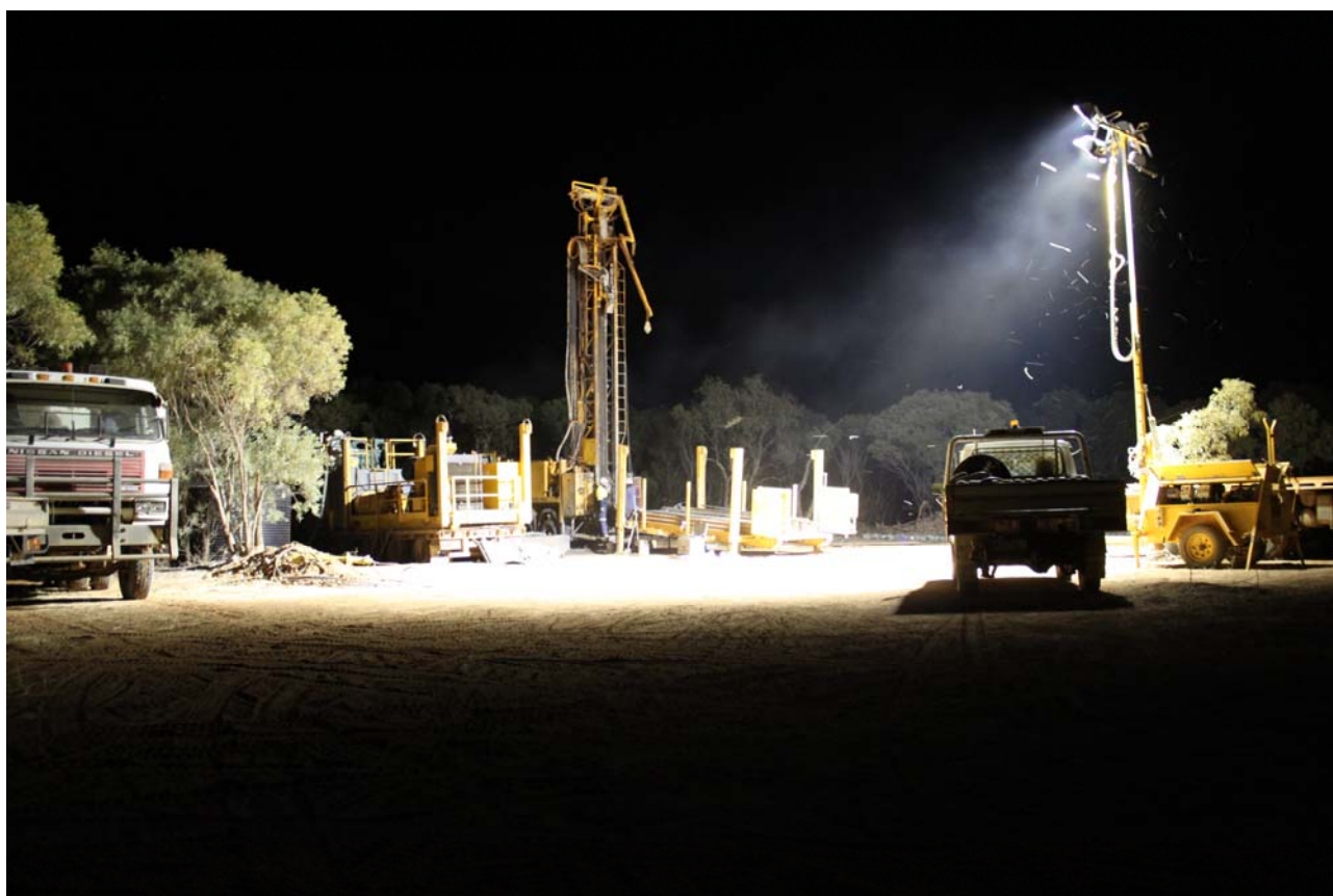
"Night shift" diamond drilling at the Gregory IOCG Project (AUGDD-01).
