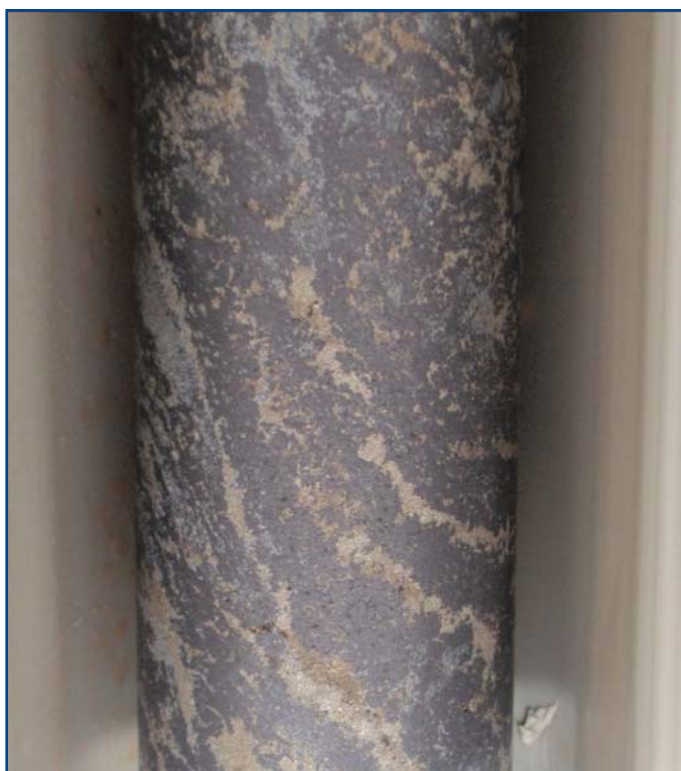
Figure 4 - Drill hole NEUDD-01 - Pervasive magnetite-pyrite alteration (759.6m).
