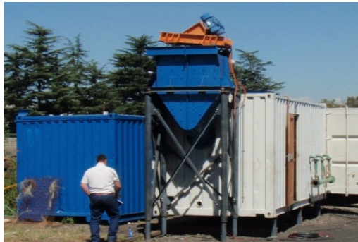
Venus Containerised Plant (above) Plant in foreground comprises hopper/feeder (blue/orange structure on frame) feeding the scrubbing/screening plant – white container 1
