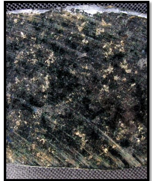
Figure 3: Ni and Cu sulfides in Mt Arrowsmith East drill core
