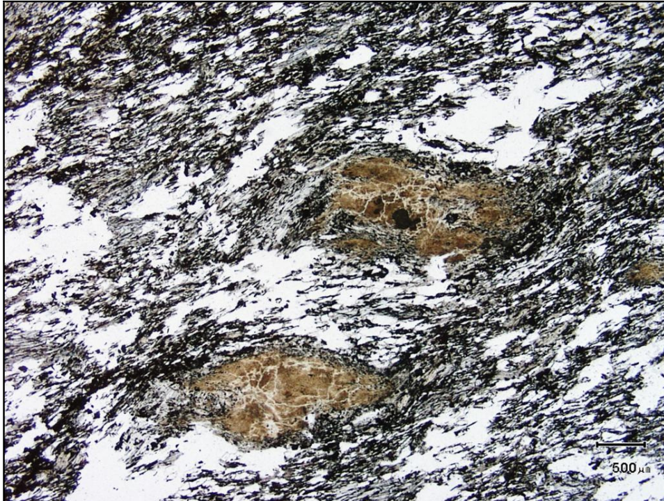
Plate 1. Transmitted light, graphite is the black mineral, scale is 500μm (0.5mm)
