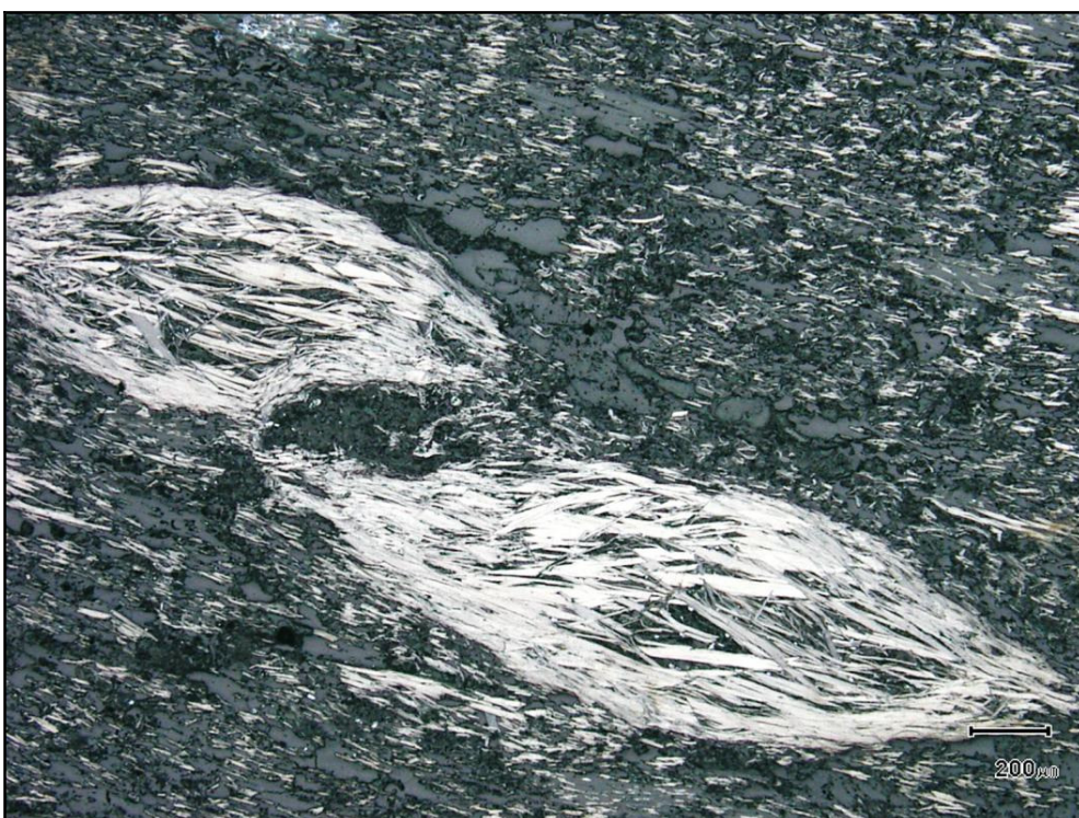
Plate 5. Reflected light, graphite clots are the white aggregates, scale is 200 \mu m (0.2mm)
