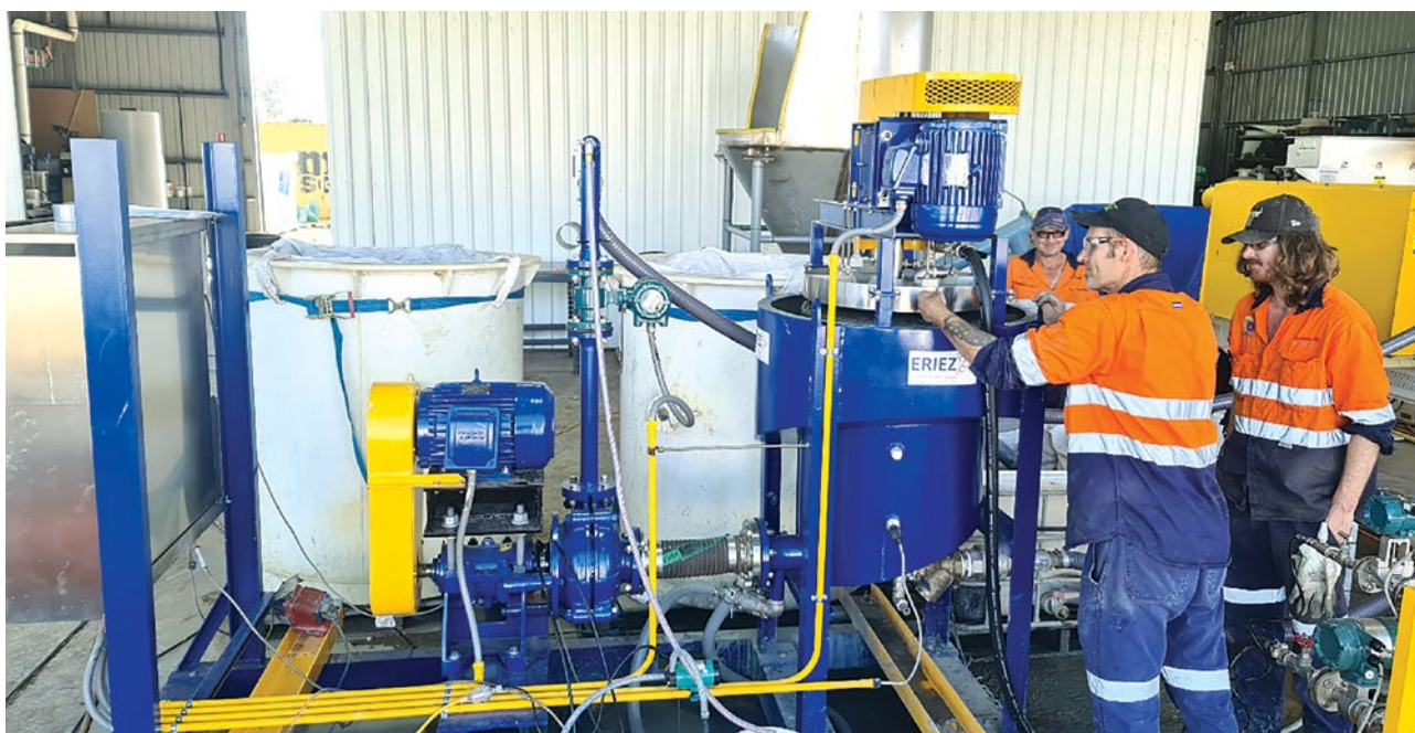
Figure 3 – Commissioning of the float cell
