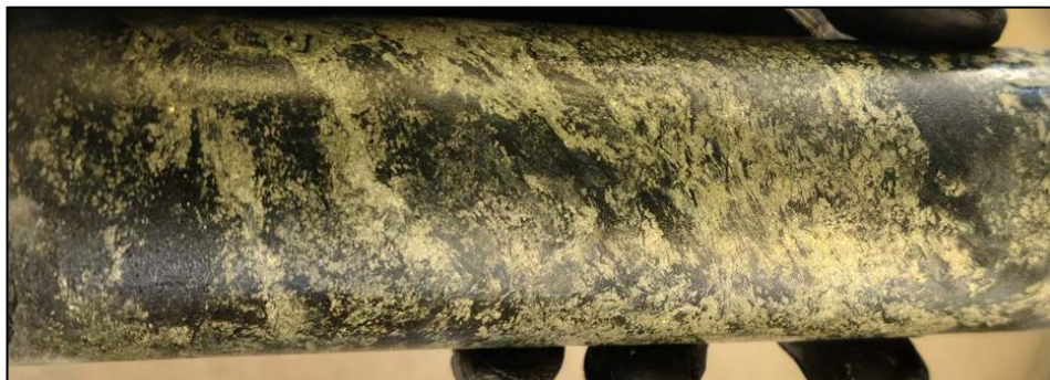
Figure 1 – Drill hole WT-21-45: semi-massive chalcopyrite (yellow copper-bearing mineral, 333.4m downhole depth)
